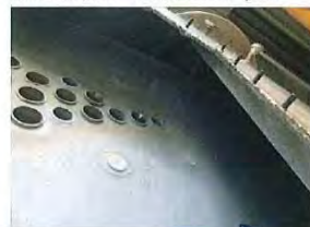
Rear end plate - smoke tube 3 rd pass
